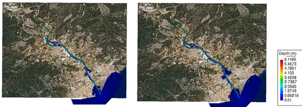
Figures 11 and 12: Simulation results showing too high of a variation between two consecutive timesteps ; t = 194400s (left) and t = 19800s (right).
