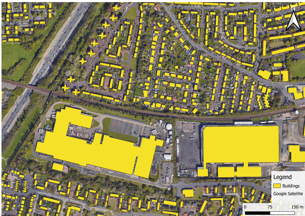
Figure 5: implementation of the buildings on HEC-RAS, visualisation from QGIS.
