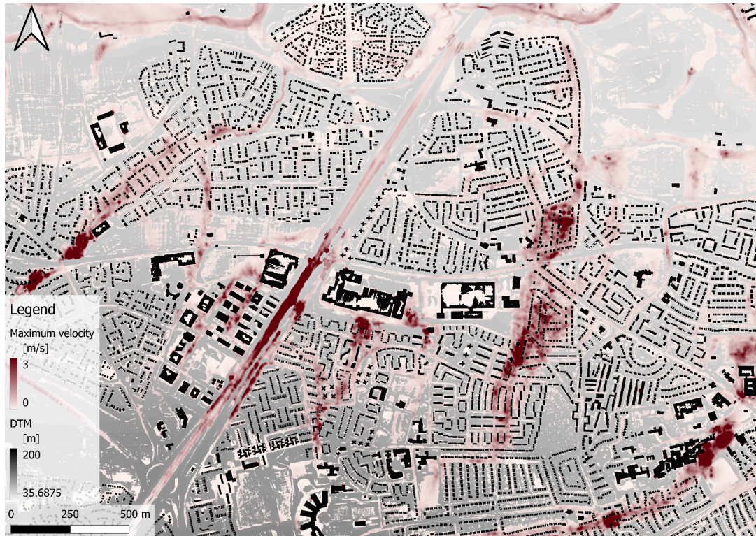
Figure 16: maximum velocity for a 100-year return period summer storm (future) on HEC-RAS, urban area.
